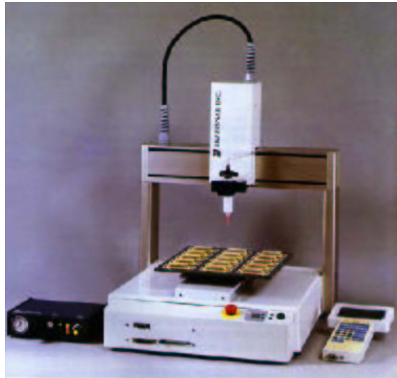
Figure 20: The Fisnar bench robot used for the application to the modules of reinforcement glue.
