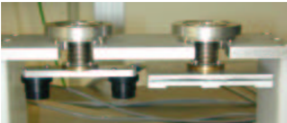
Figure 8: Photo of the hybrid (left) and sensor (right) pick-up tools on the gantry tool rack.
