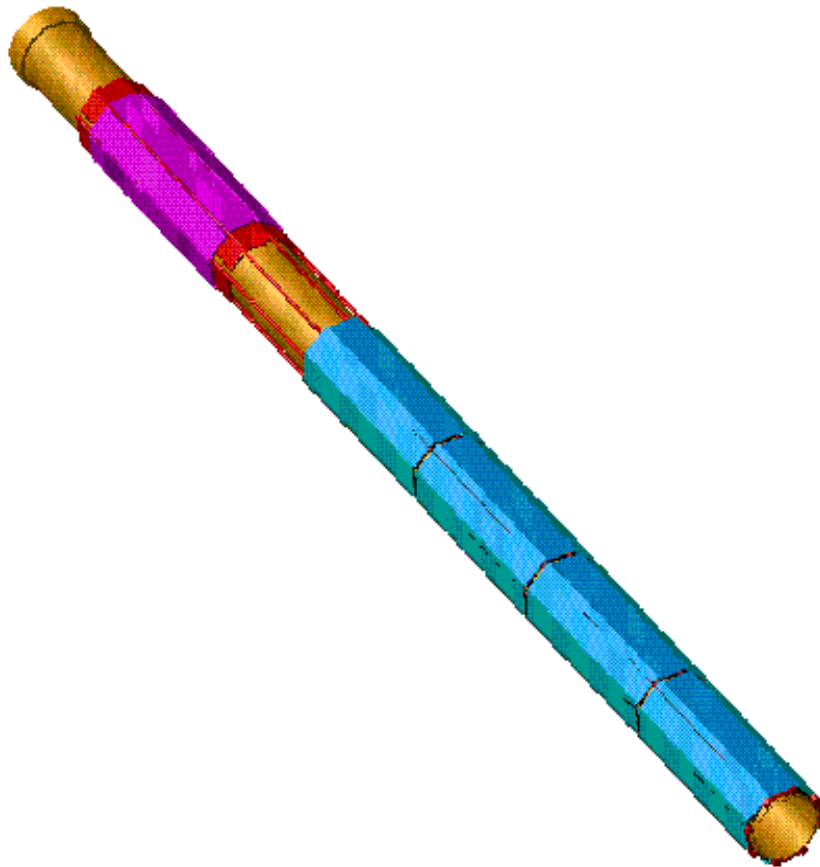
Figure 9. Solid model rendering of one half of Layer 00. Shown are 4 sensor groups (blue) starting at z = 0 , and the hybrids (magenta) starting at z \sim 45 cm.
