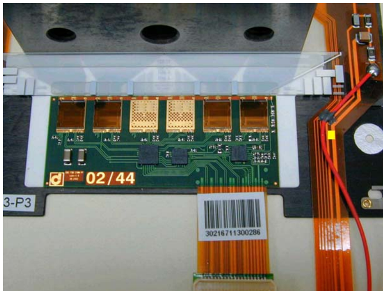
Diagram 4: Ideal location of the HV wire glue point.
