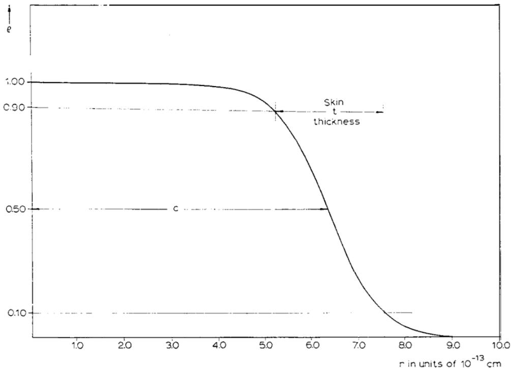
Fig. 7. The shape and parameters which describe an approximate model of the gold nucleus. This type is called the Fermi model<sup>9</sup>.
