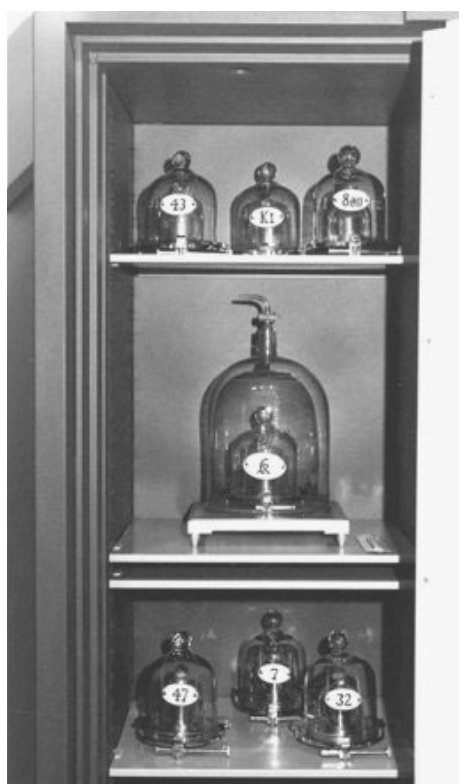
Figure 3. The international prototype and its six official copies in the safe used since the end of the third periodic verification.
