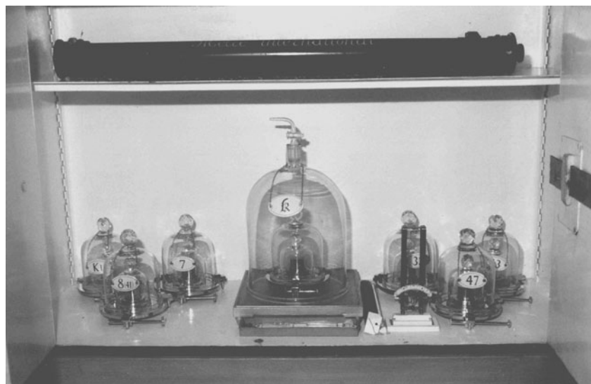
Figure 2. The international prototype of the kilogram and its six official copies. This safe was used until the end of the third periodic verification. The original international prototype of the metre is stored in the black tube on the upper shelf.
